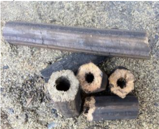
Industrial size briquettes from human waste and saw dust
