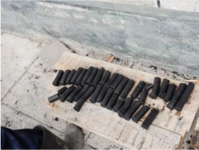
Briquettes made of carbonised human waste
